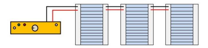
Figure 2. Frames connected parallel to pulse generator
